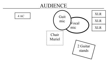
NOTE:. Both stands coming from her right or low reaching up to leave left hand free. Best visually if guitar mic stand is low with boom Guitar mic should be pointed at the  $14^{th}$  fret. Direct boxes (XLR) and power outle (AC) may be to the front or to the rear of the performer.
